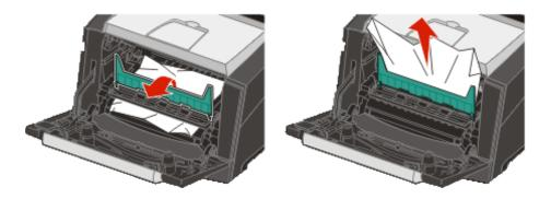
7 Open the rear exit, and remove the jammed pages.
