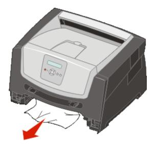
**3** Press down on the green duplex flap to release jammed pages from the duplex area, and then remove any crumpled paper.
