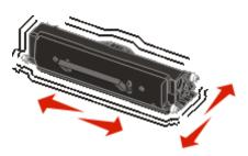
6 Install the new toner cartridge by aligning the white rollers on the toner cartridge with the white arrows on the tracks of the photoconductor and pushing the toner cartridge in as far as it will go. The toner cartridge *clicks* into place when correctly installed.
