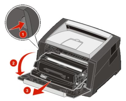
3 Lift the green flap at the front of the printer, and then remove the jammed pages beneath the flap.
