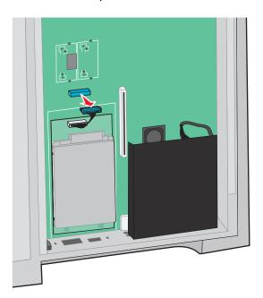
**b** Remove the screws that secure the hard disk.
