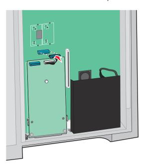
**8** Remove the thumbscrews that attach the hard disk mounting bracket to the hard disk, and then remove the bracket.
