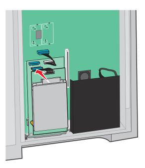
**13** Secure the hard disk to the system board cage.
