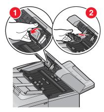
**3** Unpack the new separator pad, and then install it in the scanner.
