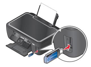
Bluetooth Dongle Connected appears on the display.
