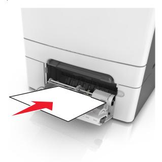
**4** Slide the paper guide until it lightly rests against the edge of the paper stack.
