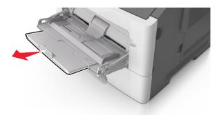
**b** Pull the extender gently so that the multipurpose feeder is fully extended and open.
