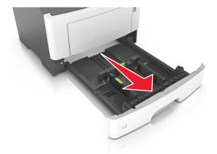
2 Squeeze and then slide the width guide tab to the correct position for the size of the paper you are loading.
