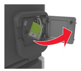
**3** Pull down the latch of the staple cartridge holder, and then pull the holder out of the printer.
