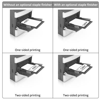
• If you are loading prepunched paper for use with the staple finisher, then make sure the holes on the long edge of the paper are on the right side of the tray.
