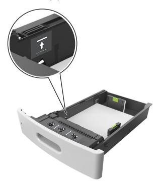
**Warning—Potential Damage:** Overfilling the tray can cause paper jams.
