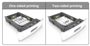
**Note:** If the holes on the long edge of the paper are on the left side of the tray, then a jam may occur.
