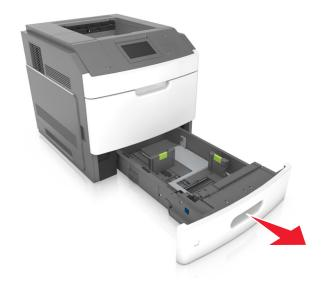
**2** Squeeze and slide the width guide to the correct position for the size of the paper being loaded until it *clicks* into place.
