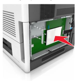
**b** Use the two provided screws to attach the printer hard disk mounting bracket.
