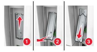
**5** Align the posts of the plastic bracket with the holes on the controller board cage, and then press the plastic bracket on the controller board cage until it *clicks* into place.
