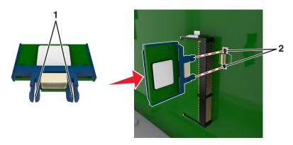
**4** Push the card firmly into place as shown in the illustration.
