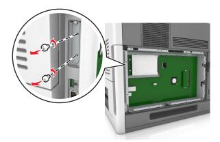
4 Remove the printer hard disk.
