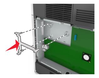
**Note:** Make sure that the plastic bracket has latched completely, and that the plastic bracket is seated firmly on the controller board cage.
