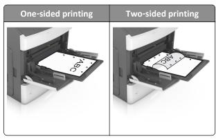
**Note:** If the holes on the long edge of the paper are on the left side of the tray, then a jam may occur.
