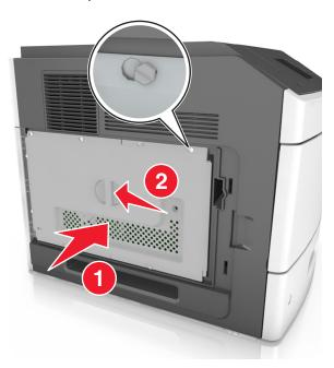
**6** Tighten the screws on the shield.
