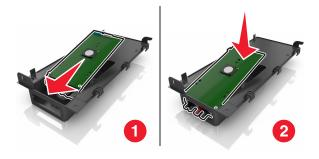
**6** Secure the ISP solution to the plastic bracket using the long screw.
