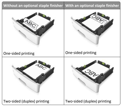
• Make sure the paper is below the maximum paper fill indicator located on the side of the width guide. Overfilling may cause paper jams.
