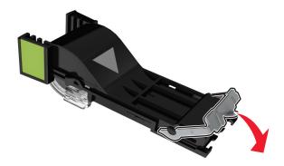
Insert staple cartridge back into the finisher until it *clicks* into place.
