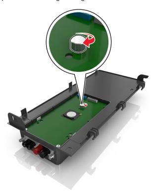
7 Tighten the two screws on the end of the ISP solution.
