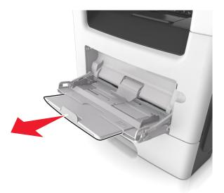
**b** Pull the extender gently so that the multipurpose feeder is fully extended and open.
