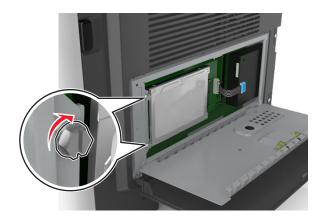
**4** Close the controller board shield, and then close the controller board access door.
