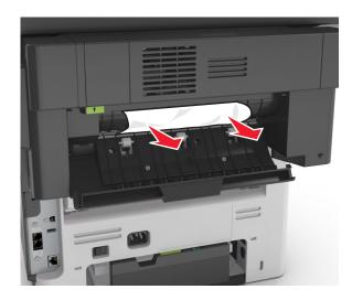
Open the finisher narrow door, and then remove any paper fragments inside the narrow door.
