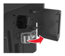
Insert the spare staple case into the staple cartridge.
