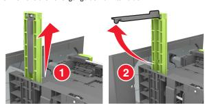
**d** Insert the A5 length guide into its designated slot.
