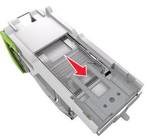
**Note:** If the staples are at the rear of the cartridge, then shake the cartridge downward to bring the staples near the metal bracket.
