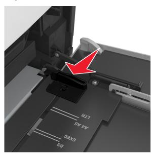
**Note:** Use the paper size indicators on the bottom of tray to help position the guides.
