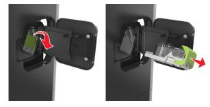
Use the metal tab to lift the staple guard, and then remove any loose staples.
