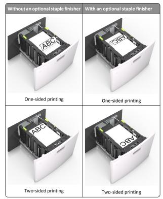
If you are loading prepunched paper for use with the staple finisher, then make sure the holes on the long edge of the paper are on the right side of the tray.
