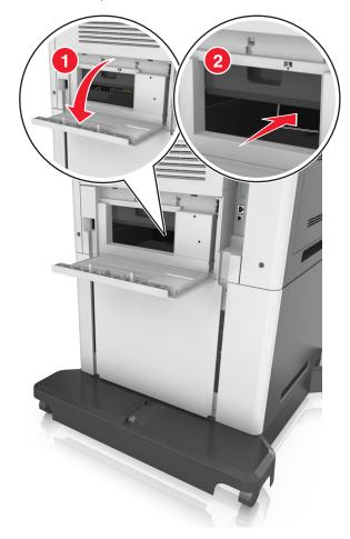
**5** Press down the rear duplex flap, then firmly grasp the jammed paper, and then gently pull the paper out.
