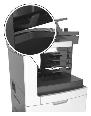
**Note:** If the paper is not under the bin arm, then a jam occurs due to an overfilled bin.
