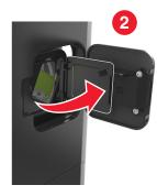
Pull down the latch of the staple cartridge holder, and then pull the holder out of the printer.
