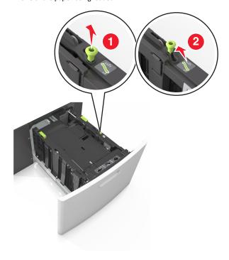
**b** If the A5 length guide is still attached to the length guide, then remove it from its place. If the A5 length guide is not attached, then proceed to step d.
