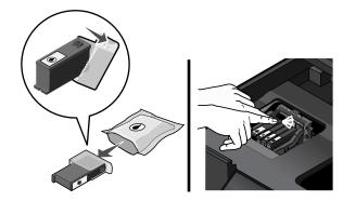
**Note:** Install the new ink cartridges immediately after removing the protective cap to avoid exposing the ink to air.
