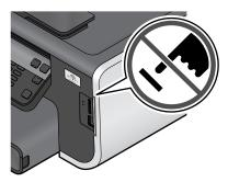
**Warning—Potential Damage:** Do not touch any cables, any network adapter, any connector, the memory device, or the printer in the areas shown while actively printing, reading, or writing from the memory device. A loss of data can occur.
