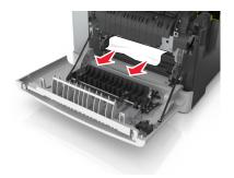
**b** Pull the green lever to open the fuser cover.
