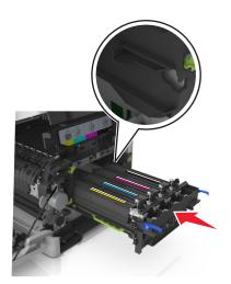
13 Gently but firmly push the blue levers down until the imaging kit fits into place.
