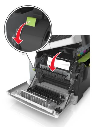
${f c}$  If there is a jammed paper in the fuser, then hold down the fuser cover, and then remove the paper.
