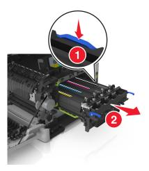
**8** Remove the used developer unit.
