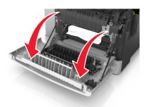
**a** If there is a jammed paper under the fuser, then firmly grasp the paper on each side, and then gently pull it out.
