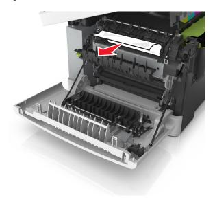
4 Slide and hold the release latch on the right side of the printer, and then slowly close the top door.
