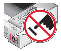
When the printer detects the memory card, the message **Memory Card Detected** appears on the control panel display.
