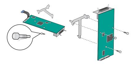
Use the provided screw to attach the ISP solution to the system board cage.
