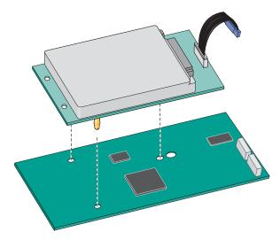
**d** Insert the plug of the printer hard disk interface cable into the receptacle of the ISP.
