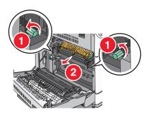
3 Lift the green lever, firmly grasp the paper on each side, and then gently pull it out.
