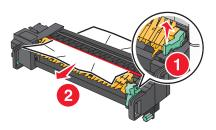
**4** Align the fuser unit using the handles on each side, and then place it back into the printer.
