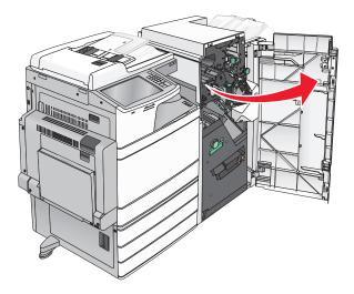
**2** Grasp the handle of the staple cartridge holder, and then pull out the holder to the right.
