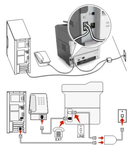
A Digital Subscriber Line splits your regular telephone line into two channels: voice and Internet. Telephone and fax signals travel through the voice channel, and Internet signals pass through the other channel. This way, you can use the same line for analog voice calls (including faxes) and digital Internet access.
