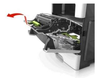
**Warning—Potential Damage:** Do not touch the shiny blue photoconductor drum under the imaging unit. Doing so may affect the quality of future print jobs.
