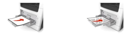
**Note:** When loading A6-size paper, make sure the multipurpose feeder extender rests lightly against the edge of the paper so that the last few sheets of paper remain in place.
