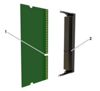
**4** Push the memory card straight into the connector, and then push the card toward the controller board wall until it *clicks* into place.
