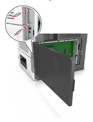
**10** Tighten the thumbscrew that is attached to the ISP.
