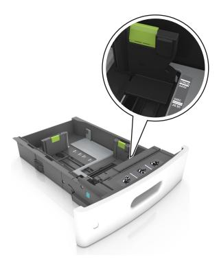
**3** Unlock the length guide, and then squeeze and slide the guide to the correct position for the size of the paper you are loading.
