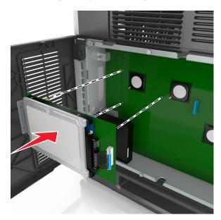
**b** Use the two provided screws to attach the printer hard disk mounting bracket.
