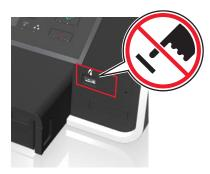
**Warning—Potential Damage:** Do not touch any cables, any network adapter, any connector, the memory device, or the printer in the areas shown while actively printing, reading, or writing from the memory device. A loss of data can occur.
