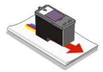
**4** Using another clean section of the dampened cloth, gently hold the cloth against the contacts for about three seconds, and then wipe in the direction shown.
