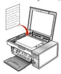
**4** Close the top cover to avoid dark edges on the scanned image.
