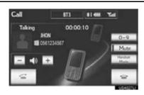
To adjust the volume of the other party's voice: Select "-" or "+", turn the "PWR·VOL" knob, or use the volume switch on the steering wheel.
