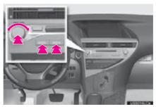
"PWR·VOL" knob: Press to turn the audio/ video system on and off. Turn this knob to adjust the volume. The system turns on in the last mode used.
