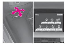
2 To select the button on the screen, press the Remote Touch knob. Once a button has been selected, the screen will change.
