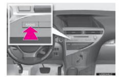
2 Select the "SAT" tab or press the "RADIO" button repeatedly until the "SAT" tab is selected.
