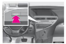
2 Select the "AM" or "FM" tab or press the "RADIO" button repeatedly to select the desired tab.
