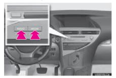
"RADIO" button: To display the "AM", "FM", "SAT" and "Apps" tabs on the screen. (Radio mode)
