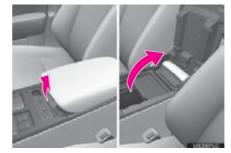
2 Open the cover and connect iPod using an iPod cable.
