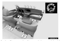
Air flows to the feet and the windshield defogger operates (Floor/windshield)
