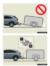
No matter which class of tow hitch applies, for a more safe trailer hookup, the trailer ball setup must be the proper height for the coupler on the trailer.
