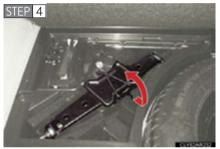
Remove the jack after removing the hook.
