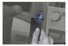
STEP 3 To change "POWER" switch modes: Within 10 seconds of the buzzer sounding, release the brake pedal and press the "POWER" switch. Modes can be changed each time the switch is pressed. (→P. 177)
