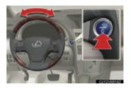
The green indicator light on the "POWER" switch will flash and a message will be shown on the multi-information display. Press the "POWER" switch again while turning the steering wheel left and right.
