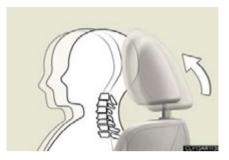
When the occupant's lower back presses against the seatback during a rear-end collision, the head restraint moves slightly forward and upward to help reduce the risk of whiplash to the seat occupant.
