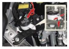
Move the washer fluid filler opening.
