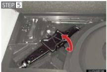
Remove the jack after removing the hook.
