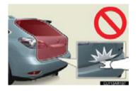
In the event that the back door is left slightly open, the back door closer will automatically close it to the fully closed position. It takes several seconds before the back door closer begins to operate. Be careful not to catch fingers or anything else in the back door, as this may cause bone fractures or other serious injuries.
