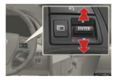
Toggle the "ENTER" switch on the steering wheel upward or downward through several items to select the energy monitor display.
