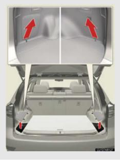
Pull the strap upwards when lifting the cover up.
