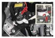
Move the washer fluid filler opening.
