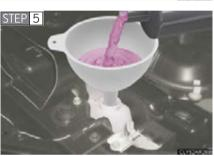
Add engine coolant if necessary.
