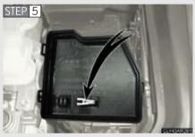
Remove the fuse with the pullout tool.
