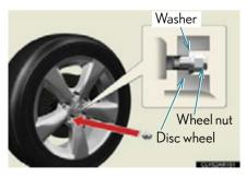
Turn the nuts until the washers come into contact with the wheel.
