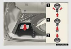
Install the 12-volt battery cover with the clips.
