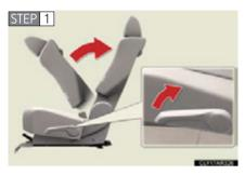
Fold the seatback while pulling the seatback angle adjustment lever. Return the seatback and secure it at the first lock position. ( $\rightarrow$ P. 86)
