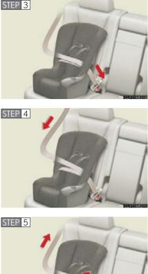
Run the seat belt through the child restraint system and insert the plate into the buckle. Make sure that the belt is not twisted
