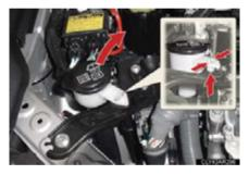
Move the washer fluid filler opening.
