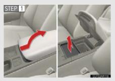
Slide the armrest while pulling up the lever, and lift the armrest. Remove the upper tray.
