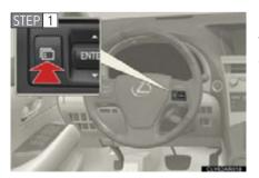
Press and hold the menu switch of the multi-information switches to display customize mode.
