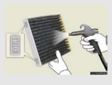
If the filter is dirty, clean by blowing compressed air through the filter from the underside.
