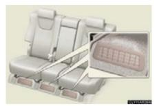
There are air intake vents under the rear seats for the purpose of cooling the hybrid battery (traction battery). If the vents become blocked, it may become the cause of malfunctions such as the hybrid battery overheating, a reduction in battery output power etc.
