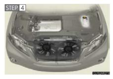
After the hybrid system has cooled down, check the power control unit coolant level and inspect the cooling system for leaks.
