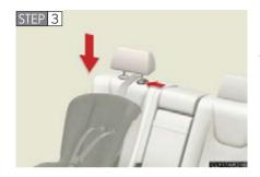
Replace the head restraint and lift it up to the uppermost lock position.
