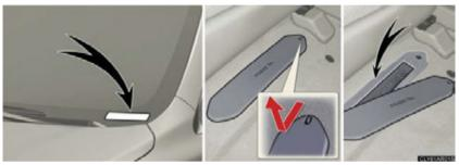
This number is stamped on the top left of the instrument panel. On some models, this number is also stamped under the front passenger seat.
