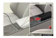
When the cover is slid open, accessory device cables can be pulled through the opening.
