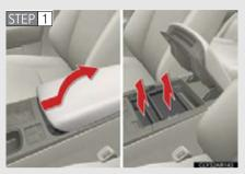
Slide the armrest while pulling up the lever, and lift the armrest. Remove the upper trays (if equipped).
