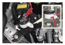
Move the washer fluid filler opening.
