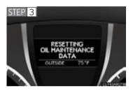
Keep the "ODO/TRIP" button pressed for about 5 seconds. The resetting procedure is complete when "OOOOOO" in the trip meter flashes once and the message in the multiinformation display disappears.
