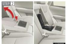
Pull up the lever to release the lock and lift the armrest.
