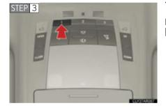
Press and hold one of the HomeLink<sup>®</sup> buttons and the transmitter button. When the HomeLink<sup>®</sup> indicator light changes from a slow to a rapid flash, you can release both buttons.
