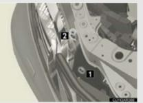
Adjustment bolt AAdjustment bolt B
