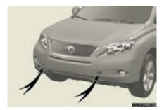
If a tow truck is not available in an emergency, your vehicle may be temporarily towed using a cable or chain secured to the emergency towing eyelet(s). This should only be attempted on hard surfaced roads for short distances at under 18 mph (30 km/h).
