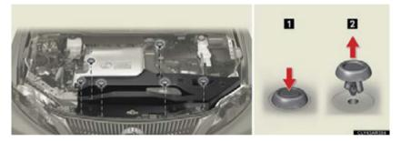
Installing the clips
