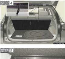
Use the hook to secure the deck board as shown in the illustration.
