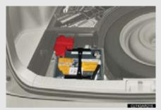
The 12-volt battery is located on the left-hand side of the luggage compartment.
