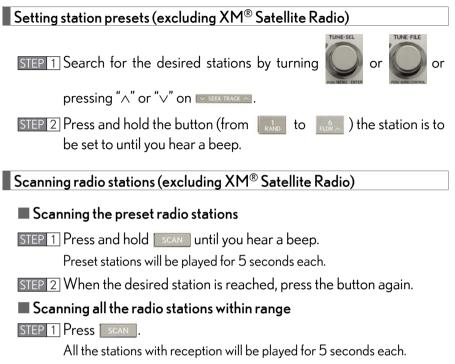
STEP 2] When the desired station is reached, press the button again.
