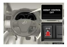
Press the height control off switch while the vehicle is stopped. A message will appear on the multiinformation display, and vehicle height will be fixed in the current mode.
