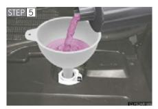
Add power control unit coolant if necessary.
