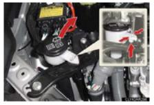
Move the washer fluid filler opening.
