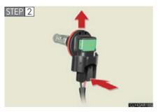
Unplug the connector while pressing the lock release. Parking lights (vehicles without LED headlights)
