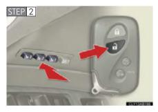
While pressing the desired button ("1", "2" or "3"), push and on the wireless remote control until the signal beeps.
