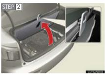
Secure the panel using the hook provided.
