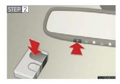
Press and hold one of the HomeLink<sup>®</sup> buttons and the transmitter button. When the HomeLink<sup>®</sup> indicator light changes from a slow to a rapid flash, you can release both buttons.
