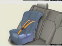
Seat belts equipped with a child restraint locking mechanism (ALR/ELR belts except driver's seat belt) (→P. 64)
