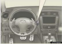
Press the "ENGINE START STOP" switch.
