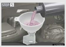
Add engine coolant if necessary.
