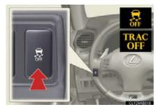
Push and hold the switch for 3 seconds or more to turn off TRAC and VSC.
