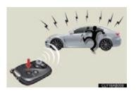
When **(1)** is pushed for longer than about one second, an alarm will sound for about 60 seconds and the vehicle lights will flash to deter any person from trying to break into or damage your vehicle.
