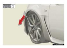
Slightly loosen the wheel nuts (one turn).
