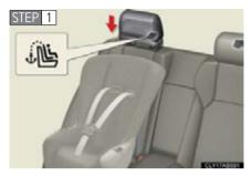
Secure the child restraint using a seat belt or the lower anchors, and lock the head restraint in place at the original position.
