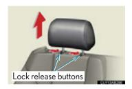
Pull the head restraint up while pushing both of the lock release buttons.
