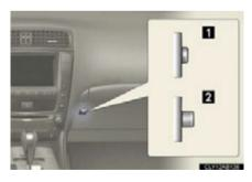
Turn the main switch in the glove box off to disable the trunk opener.
