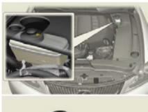
The brake fluid level should be between the "MAX" and "MIN" lines on the tank.
