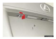
Turn the mechanical key clockwise to open.
