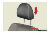
Align the head restraint with the installation holes and push it down to the lock position.
