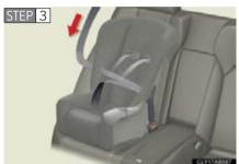
Fully extend the shoulder belt and allow it to retract to put it in lock mode.
