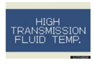
If the automatic transmission fluid temperature warning message is displayed while driving, make sure you return to normal D position driving and reduce speed by easing off the accelerator pedal. Stop the vehicle in a safe place, shift the shift lever to the P position and let the engine idle until the warning message goes out.
