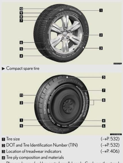
Plies are layers of rubber-coated parallel cords. Cords are the strands which form the plies in a tire.
