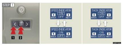
Push "<" or ">" to select the speed or tacho indicator set mode. ( $\blacksquare$ ) Turn the speed or tacho indicator to "OFF" and then "ON" by pushing the "ON/OFF" button. ( $\blacksquare$ )
