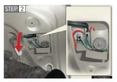
Partly remove the trunk panel cover and turn the bulb base counterclockwise.
