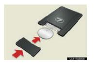
• If the battery cover is not installed and the battery falls out or if the battery was removed because the key got wet, reinstall the battery with the positive terminal facing the Lexus emblem.
