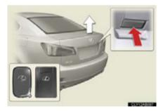
Press the button to unlock the trunk.
