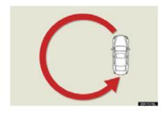
When "C" appears on the display, drive the vehicle at 5 mph (8 km/h) or less in a circle until a direction is displayed.
