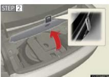
Secure the panel using the hook provided.
