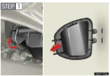
Release the lock and remove the cover.
