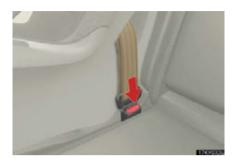
Push the buckle release button and fully retract the seat belt.
