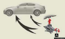
Turn the tire jack portion "A" by hand until the notch of the jack is in contact with the jack point.
