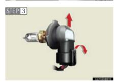
Unplug the connector while pulling the lock release.
