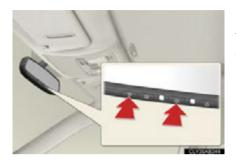
Press and hold the 2 outside buttons for 10 seconds until the indicator light flashes.
