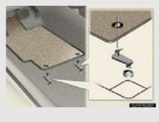
Fix the floor mat in place using the retaining hooks (clips) provided.
