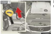
Hold a rag under the end and pull the dipstick out.
