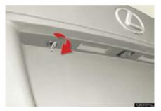
Turn the mechanical key clockwise to open.
