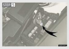
Remove the fuse with the pullout tool.
