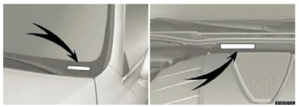
This number is stamped on the top left of the instrument panel and in the engine compartment.
