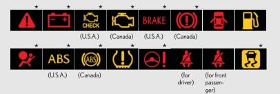
\*: These lights turn on when the "ENGINE START STOP" switch is turned to IGNITION ON mode to indicate that a system check is being performed. They will turn off after the engine is started, or after a few seconds. There may be a malfunction in a system if a light does not come on, or if the lights do not turn off. Have the vehicle inspected by your Lexus dealer.
