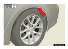
Slightly loosen the wheel nuts (one turn).
