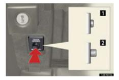
Turn the trunk opener main switch in the glove box off to disable the trunk opener.
