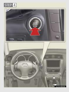
Press the "ENGINE START STOP" switch.
