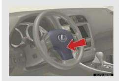
To sound the horn, press on or close to the **b** mark.
