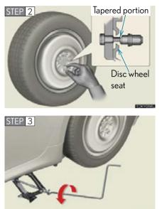
Install the spare tire and loosely tighten each nut by hand to approximately the same amount.
