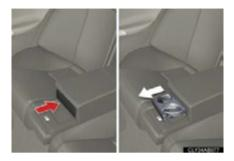
Press in and release the cup holders on the rear center armrest.
