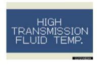
If the automatic transmission fluid temperature warning message is displayed while driving, make sure you return to normal D position driving and reduce speed by easing off the accelerator pedal. Stop the vehicle in a safe place, shift the shift lever to the P position and let the engine idle until the warning message goes out.
