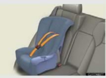
Seat belts equipped with a child restraint locking mechanism (ALR/ELR belts except driver's seat belt) (→P. 65)
