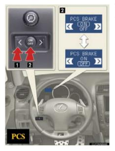
The pre-collision braking function can be turned on and off using the satellite switch.  $(\rightarrow P.348)$
