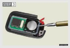
Remove the depleted battery.
