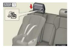
Secure the child restraint using a seat belt or the lower anchors, and lock the head restraint in place at the original position.
