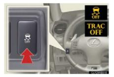
To turn the TRAC and VSC systems off, press and hold the switch for 3 seconds or more while the vehicle is stopped.
