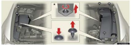
\*: Using a tool, turn the nut until the engine compartment cover can be removed.
