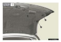
Open the trunk door and remove the cover clips.
