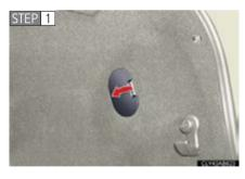
Open the trunk door and remove the cover.
