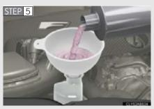
Add engine coolant if necessary.
