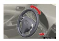
The "ENGINE START STOP" switch indicator will flash in green and a message will be shown on the multi-information display. Press the "ENGINE START STOP" switch again while turning the steering wheel left and right.
