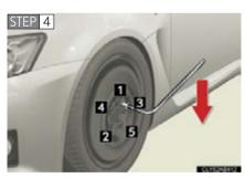
Firmly tighten each nut two or three times in the order shown in the illustration.
