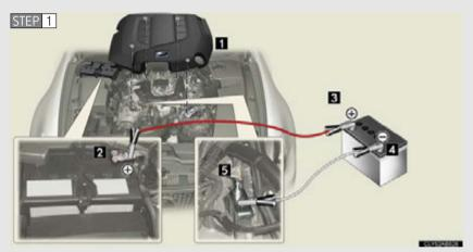
Connecting the jumper cables.
