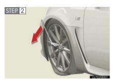
Slightly loosen the wheel nuts (one turn).
