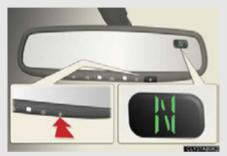
To turn the compass on or off, push the switch.
