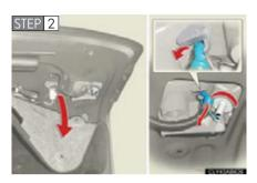
Partly remove the cover. Remove the wire harness and turn the bulb base counterclockwise.
