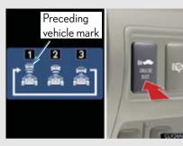
Pressing the button changes the vehicle-to-vehicle distance as follows:
