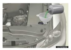
If any washer does not work or the warning message appears on the multi-information display. washer tank may be empty. Add washer fluid
