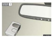
Point the remote control transmitter for the device 1 to 3 in. (25 to 75 mm) from the HomeLink<sup>®</sup> buttons.
