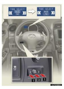
Tire pressure warning valve and transmitter ID code settings display
