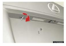
Turn the mechanical key clockwise to open.
