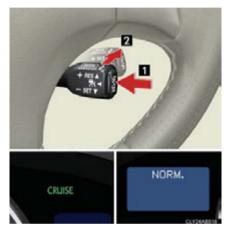
1 Press the "ON-OFF" button to activate the cruise control.
