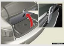
The lever can be hooked on the edge of the trunk.
