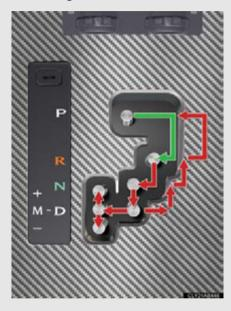
While the "ENGINE START STOP" switch is in IGNITION ON mode, depress the brake pedal and move the shift lever.
