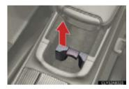
Remove the cup holder insert by holding the base part.
