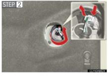
Remove the connector and turn the bulb base counterclockwise.
