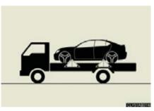
If you use chains or cables to tie down your vehicle, the angles shaded in black must be  $45^{\circ}$ .
