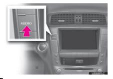
2 Touch the "SAT" tab or press the "AUDIO" button repeatedly until the "SAT" tab is selected.
