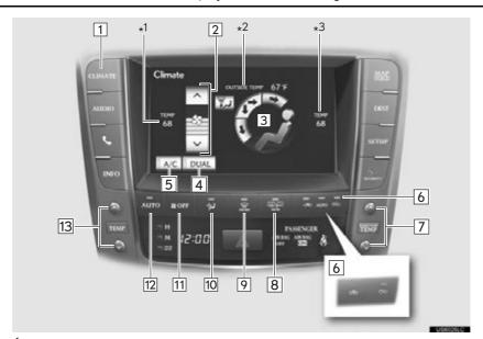
Press the "CLIMATE" button to display the air conditioning control screen.
