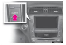
2 Touch the "AM", "FM", "SAT" or "Apps" tab or press the "AUDIO" button repeatedly to select the desired tab.
