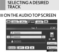
"PRSTTRACK" button: Press the ">" or "<" button of "PRSTTRACK" repeatedly until the desired track number appears on the screen. The player will start playing the selected track from the beginning.
