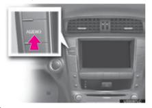
2 Touch the "iPod" tab or press the "AU-DIO" button repeatedly until the "iPod" tab is selected.
