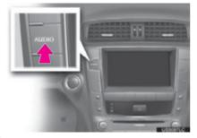
2 Touch the "BT Audio" tab or press the "AUDIO" button repeatedly until the "BT Audio" tab is selected.
