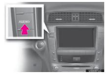
2 Touch the "USB" tab or press the "AU-DIO" button repeatedly until the "USB" tab is selected.
