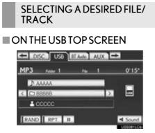
"PRSTTRACK" button: Press the ">" or "<" button of "PRSTTRACK" repeatedly until the desired file/track number appears on the screen. The player will start playing the selected file/track from the beginning.
