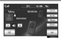
To adjust the volume of the other party's voice: Touch "-" or "+", turn the "PWR·VOL" knob, or use the volume switch on the steering wheel.
