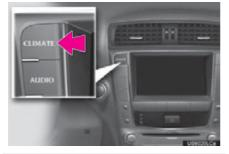
• A function that enables automatic return to the previous screen from the air conditioning control screen can be selected. See page 46 for details.
