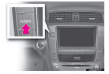
2 Touch the "DISC" tab or press the "AUDIO" button repeatedly until the "DISC" tab is selected.
