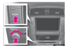
"AUDIO" button: Press to display screen buttons for the audio/video system.
