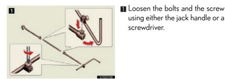
Assemble the jack handle extension bar and the jack handle bar and tighten the bolts.
