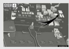
Remove the fuse with the pullout tool.
