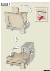
If the switch is pressed and held, the seat will automatically fold and lift sideward. (The buzzer sounds twice when the seat is about to lift.)
