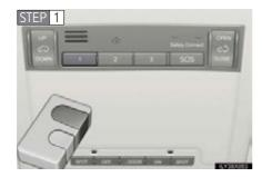
Point the remote control transmitter for the device 1 to 3 in. (25 to 75 mm) from the HomeLink<sup>®</sup> buttons.
