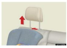
Adjust the head restraint to the upmost position.
