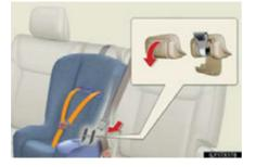
Outside only: Adjust the head restraint to the downmost position.
