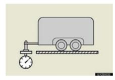
The load placed on the trailer hitch ball. ( $\rightarrow$ P. 299)
