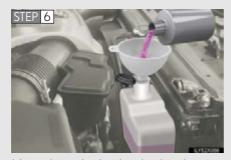
Add engine coolant if necessary.
