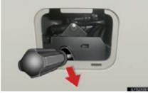
Push the lever for the back door motor, open the back door.
