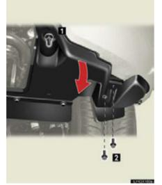
Remove the fender liner bolts, loose the fender liner nut and remove the fender liner.
