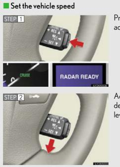
Press the "ON-OFF" button to activate the cruise control.
