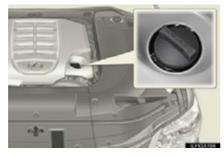
If the oil level is below or near the low level mark, add engine oil of the same type as already in the engine. ( $\rightarrow$ P. 697)
