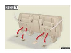
Remove the seat hook covers from the back of the seat cushion, and install them on the seat hooks.
