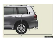
Hitch receiver pin hole position: 45.3 in. (1151 mm)
