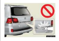
In the event that the back door is left slightly open, the back door closer will automatically close it to the fully closed position. It takes several seconds before the back door closer begins to operate. Be careful not to catch fingers or anything else in the back door, as this may cause bone fractures or other serious injuries.
