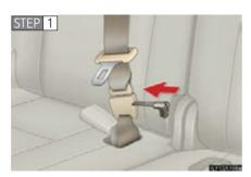
To release the hooked tab, insert the mechanical key into the hole on the buckle with the light gray buckle release button. 1 Before driving
