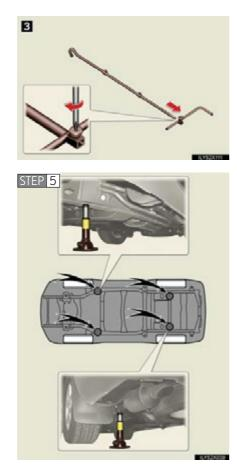
Assemble the jack handle extension bar and the jack handle and tighten the screw.
