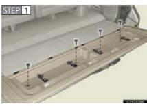
Open the back door and remove the bolts and the cover.
