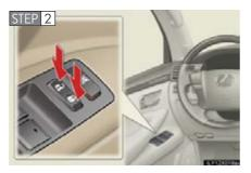
Shift the shift lever to "P" or "N", and press and hold the driver's door lock switch ( for approximately 5 seconds then release.
