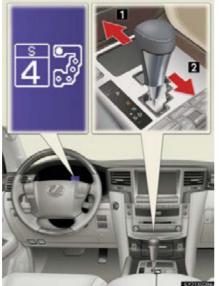
The initial shift range in "S" mode is automatically set to "5" or "4" according to the vehicle's speed. However, the initial shift range may be set to "3" or "2" if the AI-SHIFT has operated while the shift lever was in the "D" position. ( $\rightarrow$ P. 180)
