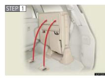
Remove the seat hook covers from the underside of the seat cushion, and install them on the seat hooks.
