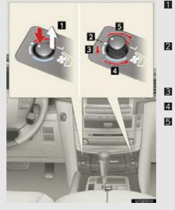
Press the knob to release it, and turn the knob to the desired temperature setting.
