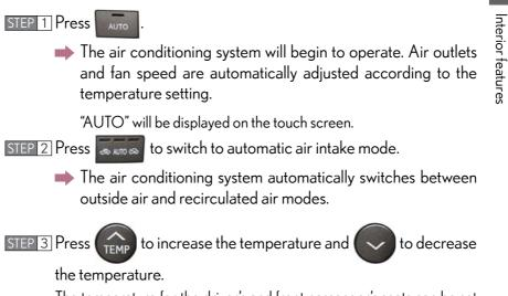
The temperature for the driver's and front passenger's seats can be set separately.
