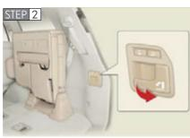
Pull the seat lock release lever and lower the seat, then lock the seat leg lock to the floor.
