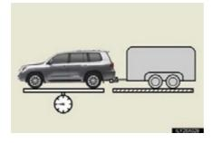
The maximum allowable gross vehicle weight. The gross vehicle weight is the total weight of the vehicle. When towing a trailer, it is the sum of the vehicle weight (including the occupants, cargo and any optional equipment installed on the vehicle) and the tongue weight.
