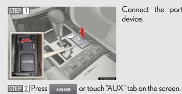
Connect the portable audio device.
