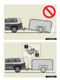
No matter which class of tow hitch applies, for a more safe trailer hookup, the trailer ball setup must be the proper height for the coupler on the trailer.
