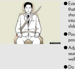
• Extend the shoulder belt so that it comes fully over the shoulder, but does not come into contact with the neck or slide off the shoulder.
