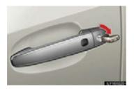
• The door is unlocked using the mechanical key.
