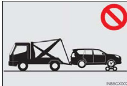
**Towing with a wheel-lift type truck**
