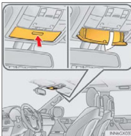
To use the overhead console when the conversation mirror is open, further extend the lid. (→P. 404)
