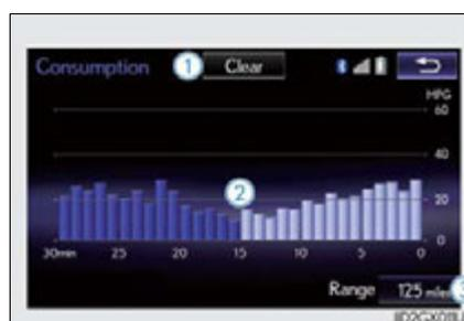
Average fuel consumption for the past 30 minutes is divided by color into past averages and averages attained since the engine switch was last turned to IGNITION ON mode. Use the displayed average fuel consumption as a reference.
