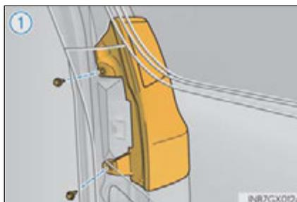
2 Close the back door half way and remove the lamp assembly.
