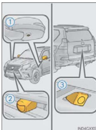
If the camera lens becomes dirty, it cannot transmit a clear image. If water droplets, snow or mud adhere to the lens, rinse with water and wipe with a soft cloth. If the lens is extremely dirty, wash it with a mild cleanser and rinse.
