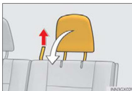
**■ Removing the head restraints****▶ Front and second seats**
