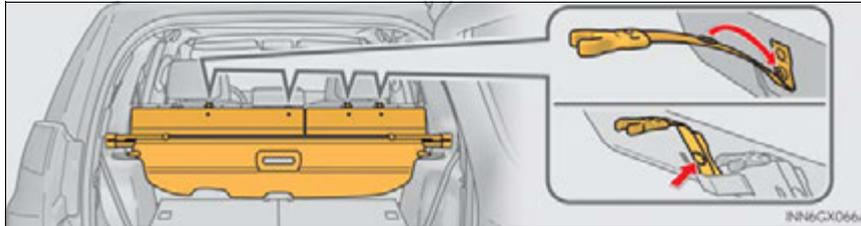
Fasten the button when the second seats are in the rear-most position.
