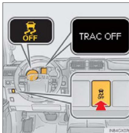
■ **When the "TRAC OFF" is displayed on the multi-information display even if the VSC OFF switch has not been pressed**
