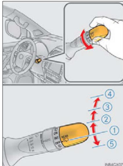
■ **The rear window wiper and washer can be operated when**
