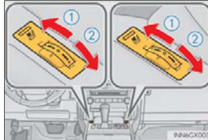
The seat heaters and ventilators can be used when the engine switch is in IGNITION ON mode.
