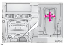
2 To select a screen button, press the Remote Touch knob or an "ENTER" button. Once a button has been selected, the screen will change.
