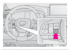
The voice command system and its list of commands can be operated. (→P.260)
