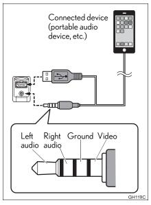
When using an iPod video, a cable that has a 4-pole AUX plug and a USB connector is necessary. Connect the plug and connector to the AUX and USB ports.
