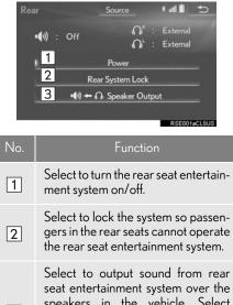
3 speakers in the vehicle. Select **"Right"** or **"Left"** to select for which screen sound will be output.  $(\rightarrow P.227)$
