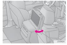
• The display angle can be adjusted between 0 degree to 50 degree.
