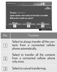
2 Check that a confirmation screen is displayed when the operation is complete.
