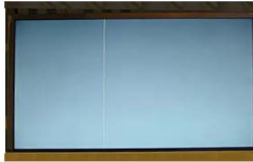
Vertical Line Source TAB IC Defect
