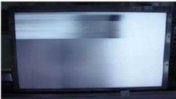
Horizontal Block Gate TAB IC Defect
