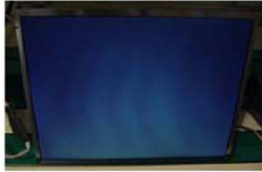
Panel Mura, Light leakage
