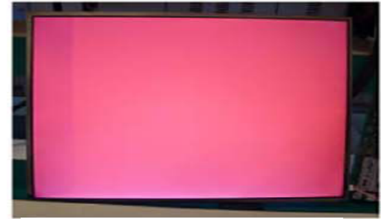
Vertical Block Source TAB IC Defect
