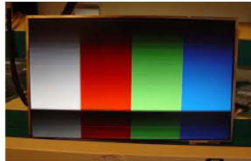
Horizontal Block Gate TAB IC Defect
