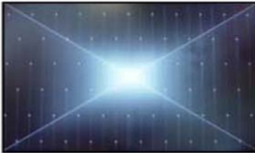
Solder defect, Short/Crack
