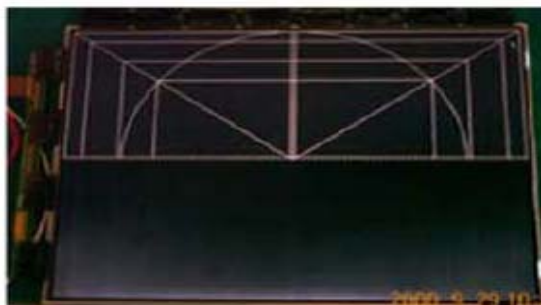
Horizontal Block Gate TAB IC Defect
