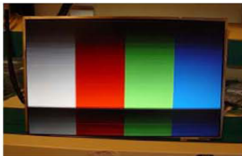
Horizontal Block Gate TAB IC Defect
