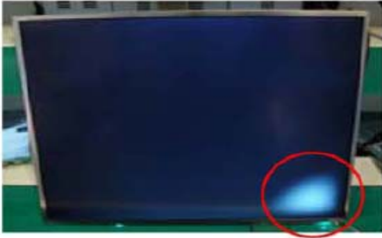
Panel Mura, Light leakage
