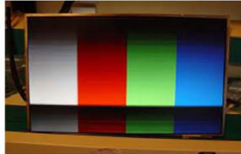
Horizontal Block Gate TAB IC Defect
