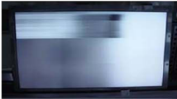
Horizontal Block Gate TAB IC Defect
