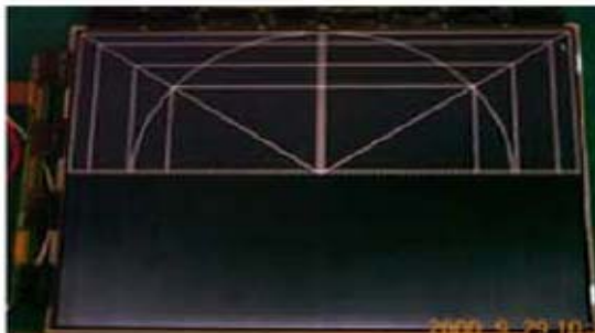
Horizontal Block Gate TAB IC Defect
