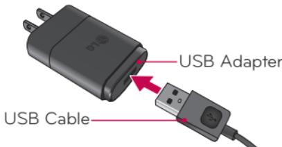
**NOTE:** Make sure the battery is installed before connecting the USB adapter. If the battery is not installed and the USB adapter is connected, the phone will not operate properly due to prolonged power cycling. Also, removing the battery with the USB adapter connected may damage the device. Please unplug USB adapter before removing battery.
