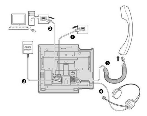
1 LAN Connect the IP Phone LAN port to the LAN wall jack with the provided LAN cable.
