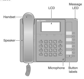
The top line of the LCD indicates a number of icons indicating the connection, status and options for the IP8815 phone. A list of the icons and there meaning are provided in <a href="Appendix C">Appendix C</a>.
