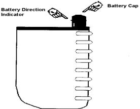
Hold the transmitter in one hand. Using the other hand thumb and index finger, grasp the battery cap and turn counter clockwise until the cap can be removed.
