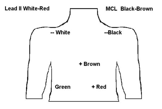
If only one lead of ECG is required remove the brown and black lead wires from the transmitter. Refer to the section on **MULTI-VIEW WAVEFORMS** in the central station operating manual to disable lead fault on second channel.
