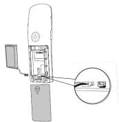
**Note:** The jack is keyed so that the plug can only be inserted in one direction. Be careful not to crimp wire.
