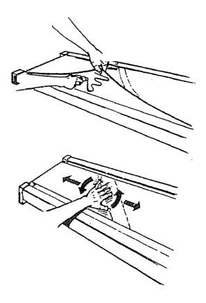
GENERAL CLEANING: Keep the unit clean by dusting regularly. The belt may be washed with a wet, soap cloth. Be caref not to get any liquid inside the Motorized Treadmill frame.
