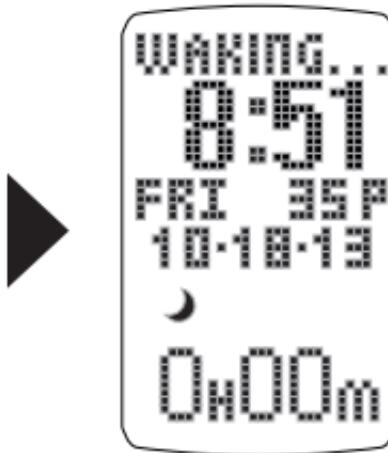
Waking screen appears when movement is sensed and the tracker is determining if you are awake.
