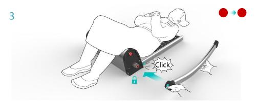
Push the rear leg (marked red for left-hand side) onto the shaft and click into place.
