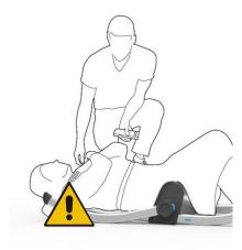
Be aware of the positioning of the shoulders and make sure that the arms are crossed upon the chest, due to the fact that the rear legs move down towards the floor as soon as the up button is pressed. This may put the person's shoulders and arms at risk of injury if not positioned correctly.
