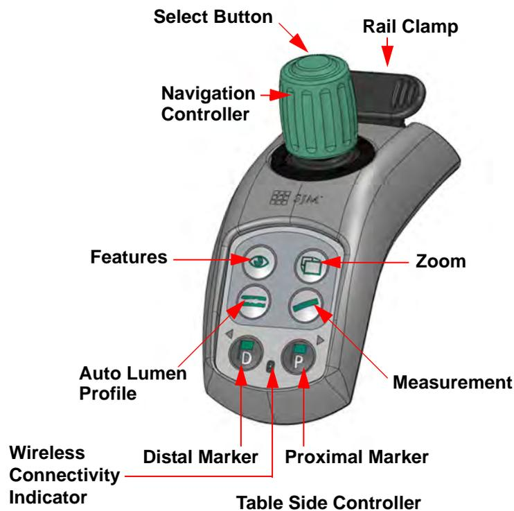
**Table Side Controller:** The TSC may be used to position the mouse cursor by moving the **Navigation Controller** to left, right, up, or down. The **Select** button (on the top of the Navigation Controller) functions as the left mouse button, and a twist of the **Navigation Controller** functions as the mouse scroll wheel (twist left is scroll up and twist right is scroll down).
