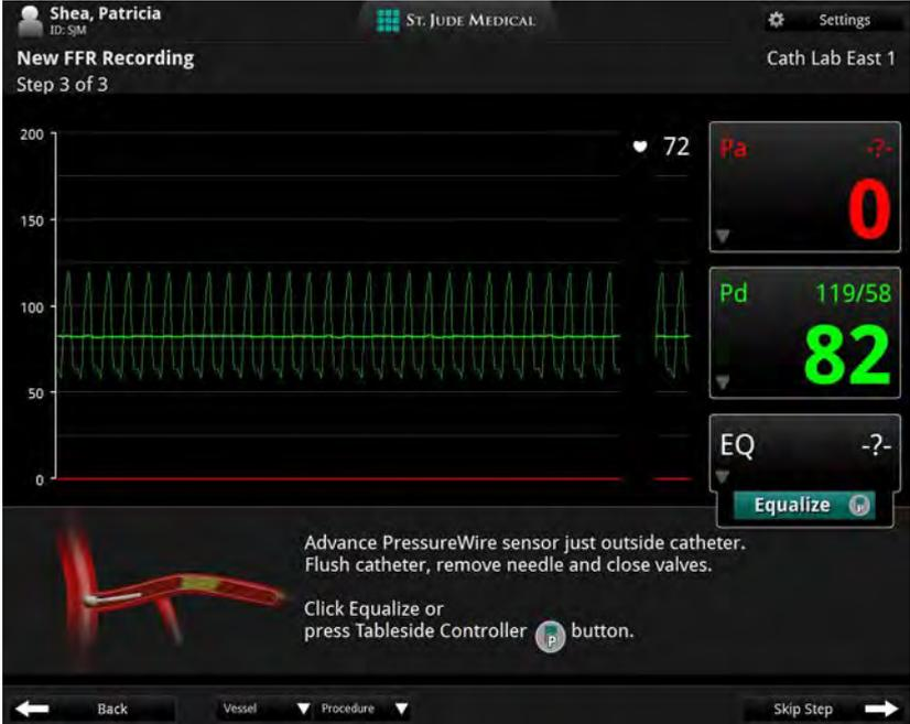
Figure 4-6: Advance PressureWire and Equalize guidance message
