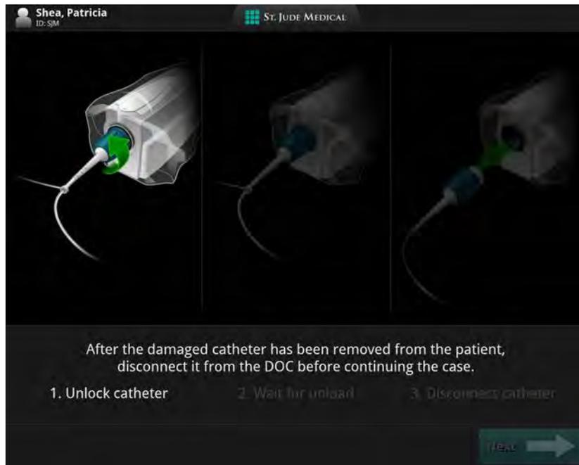
Figure 5-11: Safe Unload Guidance, Screen 1
