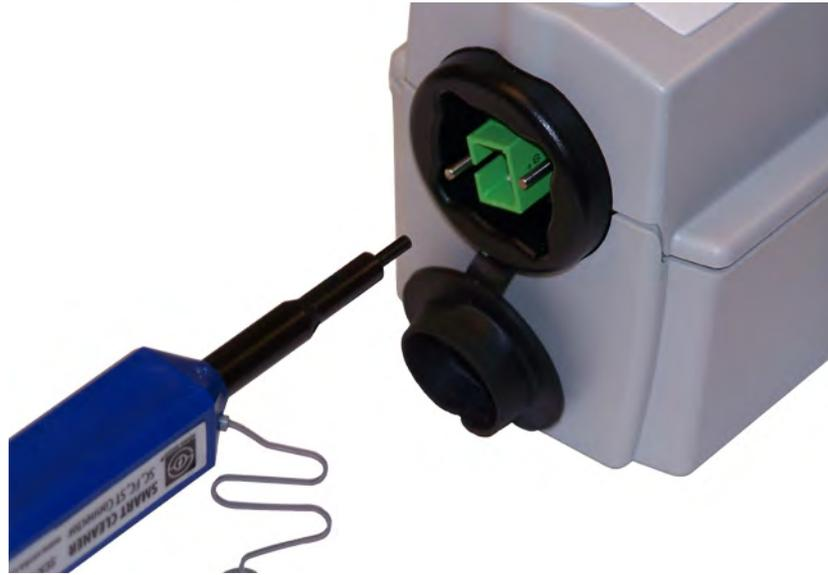
Figure 9-1: Inserting Cleaner Into Optical Adapter
