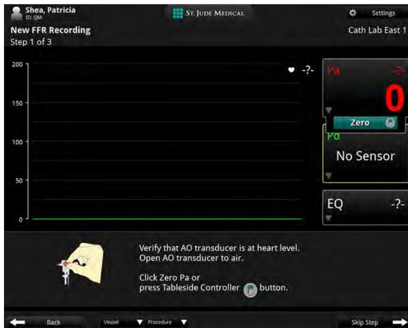
Figure 4-3: Set AO transducer height and open AO transducer guidance message
