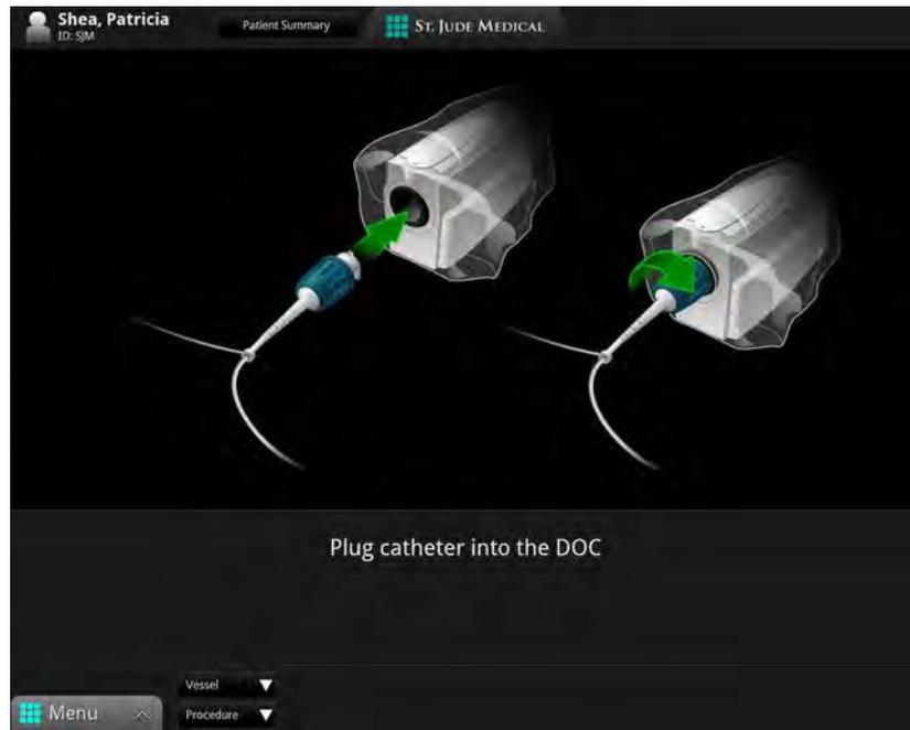
Figure 5-3: Plug Catheter into DOC Guidance Message
