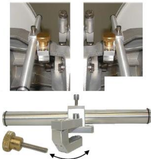
Figure 5-13: Re-configuring Alignment Sight Tool
