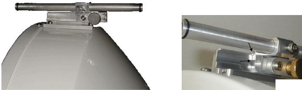
Figure 5-12: Attach Alignment Sight Tool to external 2 foot antenna
