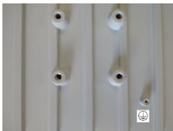
Figure 3-5: Enclosure Ground Connection
