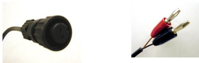
Figure 1-11: RSSI alignment cables
