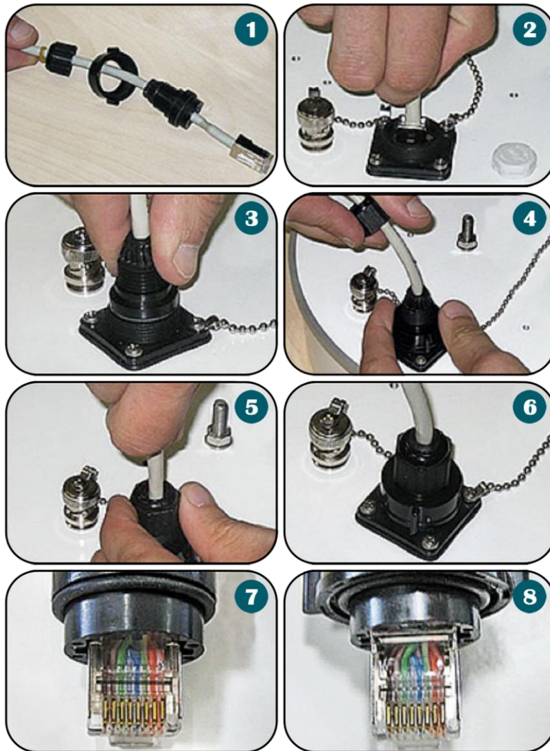
Figure 7 – Assembling Ethernet weatherproof connector
