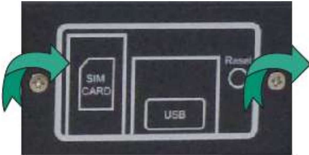
Figure 4-5 – Replace SIM/USB/Reset Panel Cover
