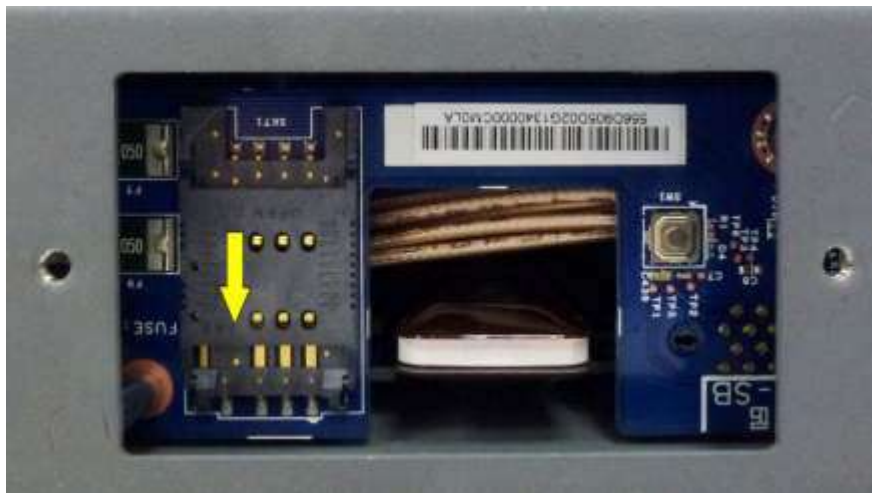
Figure 4-6 – Slide SIM Card Slot Protective Cover Down
