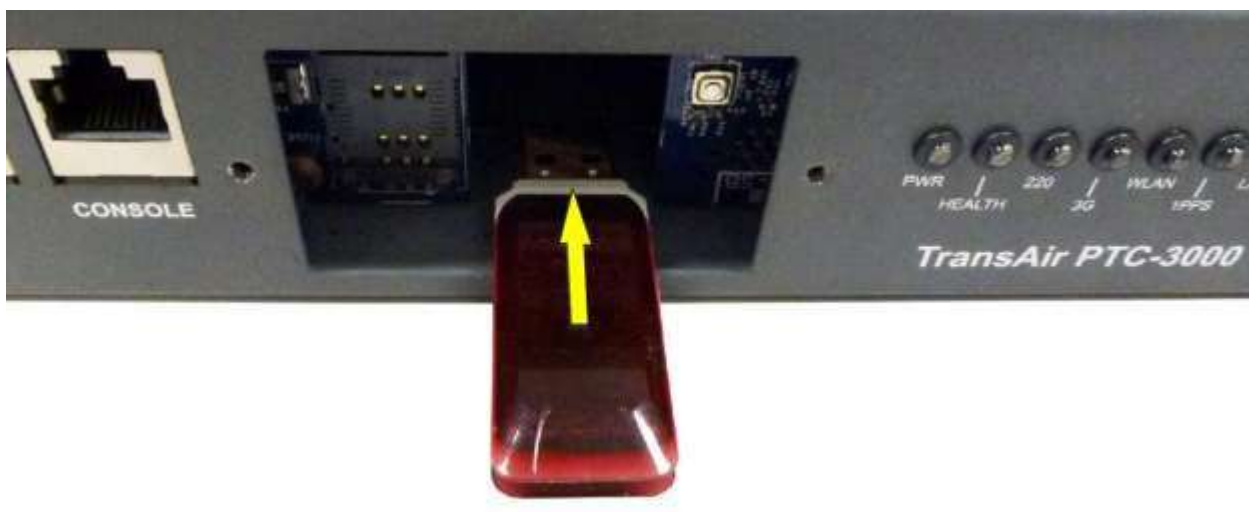
Figure 4-4 – USB Flash Drive Installation (1U unit shown)
