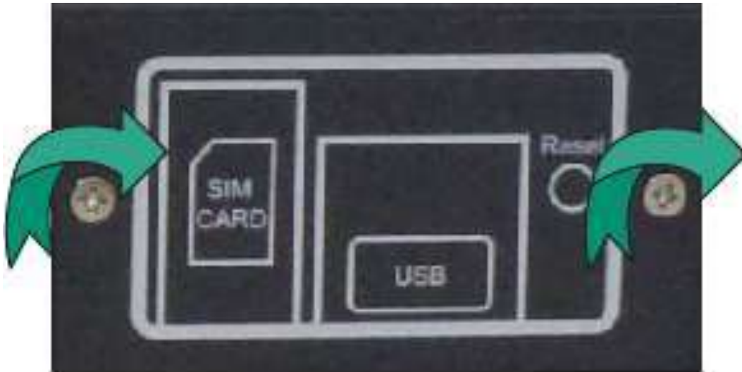
Figure 4-5 – Replace SIM/USB/Reset Panel Cover
