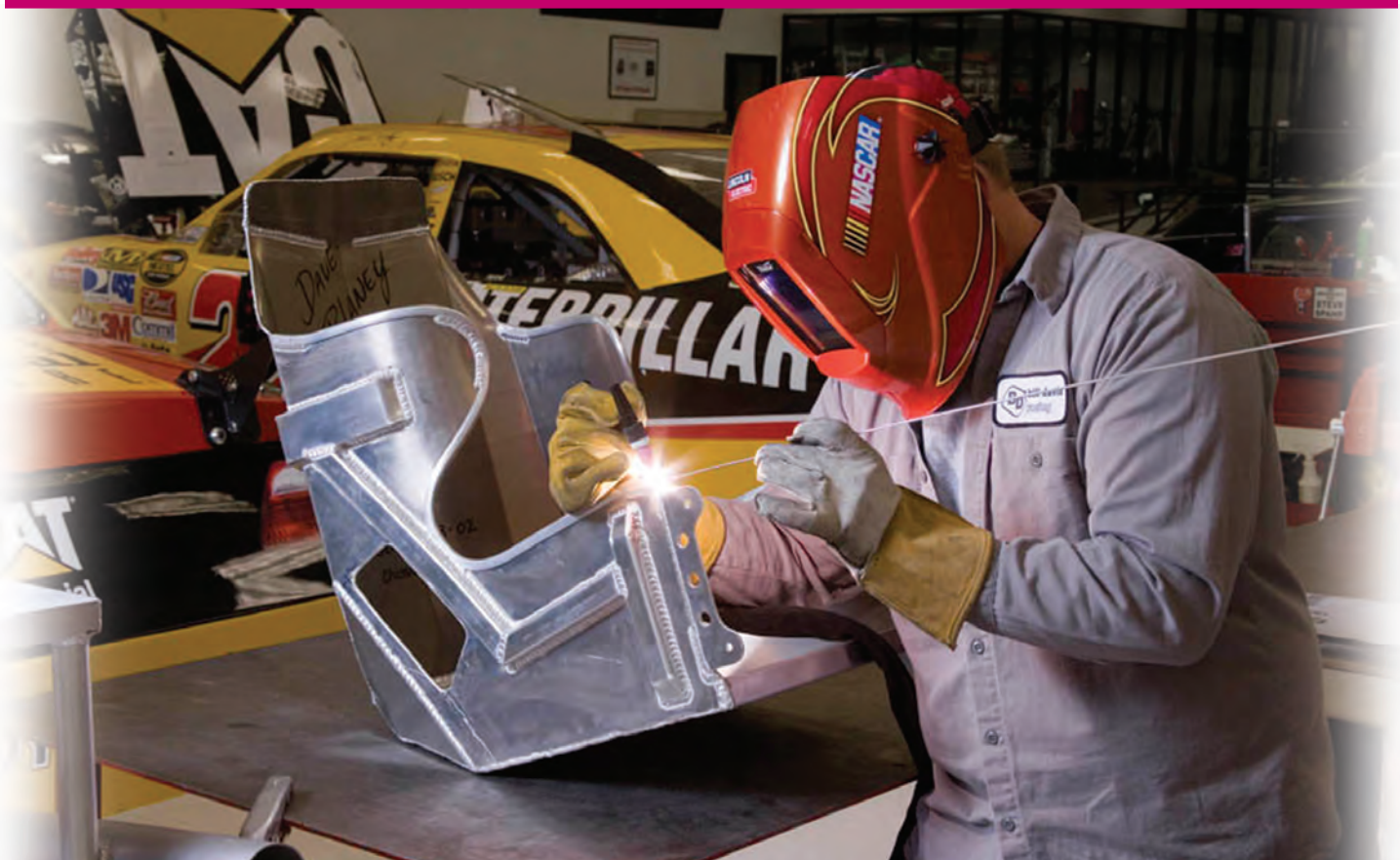
A fabricator from Bill Davis Racing® TIG welds a seat for a NASCAR® racecar using Lincoln® machines and consumables.
