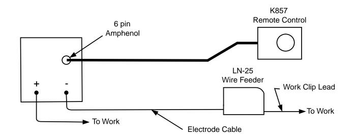
NOTE: Illustration shows electrode connected for negative polarity.
