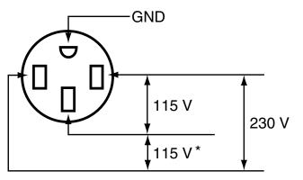
\* Current Sensing for Automatic Idle (Receptacle viewed from front of machine.)
