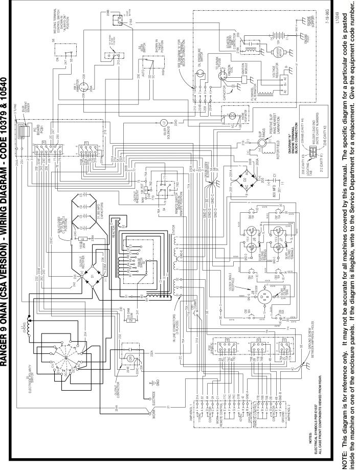
RANGER 9 ONAN (CSA VERSION) - WIRING DIAGRAM - CODE 10379 & 10540
