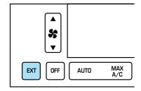
If a manual override function is selected while the outside temperature is displayed, the new function will be displayed for four seconds after it is changed, then the outside temperature will return to the window along with the override selection.
