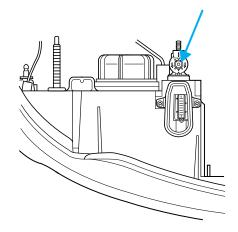
3. Use a 4 mm wrench or socket to turn the horizontal adjusting screw until the "0" mark on the yellow dial lines up with the reference mark on the marker (as shown) when viewed directly from above.
