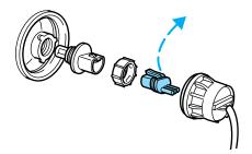
6. Remove the bulb retaining ring by rotating it counterclockwise.
