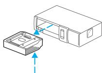
1. Pull the lever to remove a CD tray from the magazine.
