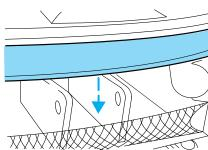
4. Lower the bracket and module tray assembly.
