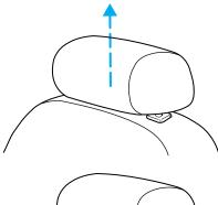
Push control to lower head restraint.
