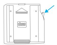
2. Insert one disc into each CD tray of the magazine (up to 6 discs). Ensure that the label side is facing up.
