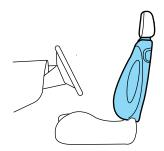
If the side air bag has deployed, the air bag will not function again. The side air bag system (including the seat) must be inspected and serviced by a qualified technician in accordance with the vehicle service manual. If the air bag is not replaced, the unrepaired area will increase the risk of injury in a collision.
