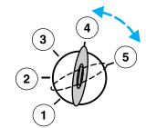
press the accelerator all the way to the floor and hold. Turn the key to the START position.
