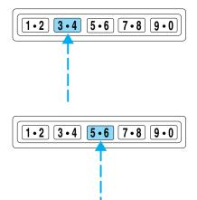
To release the trunk, enter the factory-set code or personal code (driver door unlocks) and press 5/6 within 7.5 seconds.
