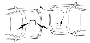
1. Connect the positive (+) booster cable to the positive (+) terminal of the discharged battery.
