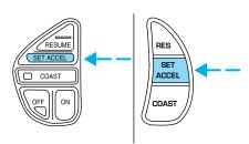
You can accelerate with the accelerator pedal at any time during speed control usage. Releasing the accelerator pedal will return your vehicle to the previously programmed set speed.
