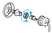
7. Remove the old bulb from the lamp assembly by pulling it straight out of the lamp assembly.
