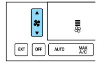
fan speed. Press the steering wheel control (if equipped) up for higher fan speed or down for lower fan speed.
