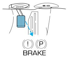
Always set the parking brake fully and make sure the gearshift is latched in P (Park). Turn the ignition to the LOCK position and remove the key whenever you leave your vehicle.
