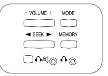
When the rear seat controls are activated, rear seat passengers can use the controls to change the playing media for all passengers (Single Play mode). In this mode, all speakers will play audio from the same media source for all passengers to hear. To activate the rear seat radio controls:
