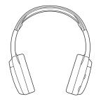
To install the batteries, lightly press down on the top of the left earpiece and slide the cover off.
