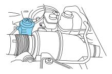
4. Check the fluid level in the reservoir. It should be between the MIN and MAX lines. Do not add fluid if the level is in this range.
