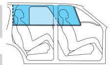
If the Safety Canopy<sup>(10)</sup> system has deployed, the Safety Canopy<sup>(10)</sup> will not function again unless replaced. The Safety Canopy<sup>(10)</sup> system (including the A, B and C pillar trim) must be inspected and serviced by a qualified technician in accordance with the vehicle service manual. If the Safety Canopy<sup>(10)</sup> is not replaced, the unrepaired area will increase the risk of injury in a collision.
