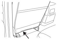
To remove climate controlled seat air filter:
