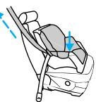
8. Allow the safety belt to retract to remove any slack in the belt.
