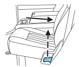
Reclining the seatback can cause an occupant to slide under the seat's safety belt, resulting in severe personal injuries in the event of a collision.
