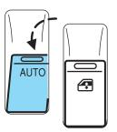
• Pull up (to the first detent) and hold the top portion of the switch to close.
