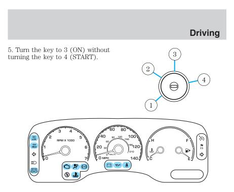
Make sure the corresponding lights illuminate or illuminate briefly. If a light fails to illuminate, have the vehicle serviced.
