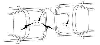
2. Connect the other end of the positive (+) cable to the positive (+) terminal of the assisting battery.
