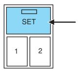
position. Press the SET control. The SET control indicator light will briefly illuminate. While the light is illuminated, press control 1.
