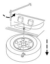
5. To remove the spare tire, turn the handle counterclockwise until the tire is lowered to the ground and the cable is slightly slack.
