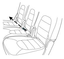
2. With the latch released the seatback can be lowered into the load floor position.
