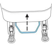
Note: This seat can be moved forward to keep a child in a child restraint close to the front seat occupants. The seat should be moved to the full rearward position when it is occupied by older children or adults.
