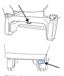
3. Route the child safety seat tether strap under the head restraint (outboard seats) and over the back of the seat.
