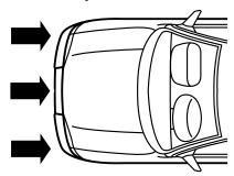
cause activation. The driver and passenger airbags are designed to inflate in frontal and near-frontal collisions, not rollover, side-impact, or rear-impacts unless the collision causes sufficient longitudinal deceleration.
