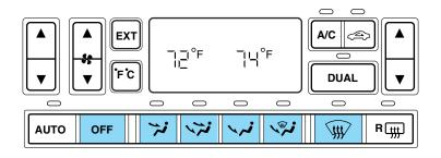
The manual override controls allow you to determine where airflow is directed. To return to full automatic control, press AUTO.
