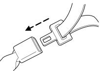
2. To unfasten, push the release button and remove the tongue from the buckle.
