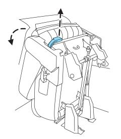
2. Pull up on the handle located at the back of the seat. The seat will flip forward.
