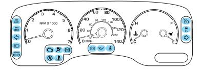
Warning lights and gauges can alert you to a vehicle condition that may become serious enough to cause expensive repairs. A warning light may illuminate when a problem exists with one of your vehicle's functions. Many lights will illuminate when you start your vehicle to make sure the bulb works. **If any light remains on after starting the vehicle, have the respective system inspected immediately.**
