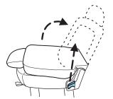
The rear latch hooks must be properly engaged with the floor striker. Position the rear legs of the seat over the floor strikers and engage.
