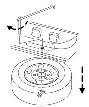
wrench will become harder to turn and the spare tire winch will ratchet or slip when the tire is raised to maximum tightness. A clicking sound will be heard from the winch indicating that the tire is properly stowed.
