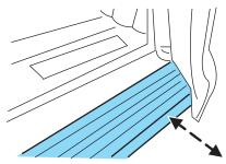
Turn off the running boards before jacking or placing any object under the vehicle. Never place your hand between the extended running board and the vehicle. A moving running board may cause injury.
