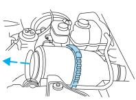
3. Remove the air filter element from the air filter housing.
