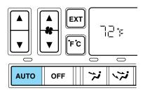
However, until the engine is warmed, the fan speed will operate at a low speed and airflow will be directed to the windshield defroster ducts. Upon engine warm up, the system will automatically direct airflow to the floor ducts and operate at the required fan speed to achieve the selected temperature.
