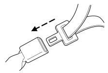
2. Grasp the shoulder portion and pull downward until the entire belt is pulled out.
