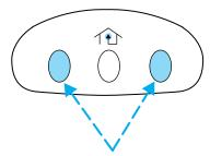
2. Position the end of your hand-held transmitter 2–8 cm (1–3 inches) away from the HomeLink<sup>®</sup> Universal Transceiver surface (located on your visor) while keeping the red light in view.
