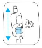
Move lock control up to engage the childproof lock. Move control down to disengage childproof locks.
