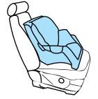
2. Pull down on the shoulder belt and then grasp the shoulder belt and lap belt together.
