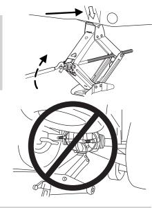
To lessen the risk of personal injury, do not put any part of your body under the vehicle while changing a tire. Do not start the engine when your vehicle is on the jack. The jack is only meant for changing the tire.
