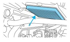
• It can be accessed from the second row seat. Move the front seat all the way forward and up to ease access.
