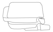
3. To return the seat to the upright position, lift the seatback until the latch is fully engaged.
