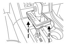
4. Press and hold the white button located along side the shifter housing assembly (as shown in the illustration). Press the gearshift lever release on the shifter knob and move the gearshift lever back to N (Neutral) (two places rearward from P [Park]).
