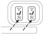
Push the top of the control button to return the seatback to its original position.
