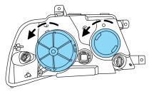
6. Once the bulb covers are removed, the bulbs can be removed by turning them counterclockwise and then pulling the bulbs straight out.
