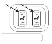
The power folding seats are designed to stall within 1-10 seconds of encountering an obstruction when opening or closing. Should this occur, remove the obstruction and wait approximately 1-4minutes for the seat motor to reset.
