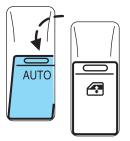
DOWN event, the window will stop. If, after 1/2 second the switch is still held, the window will perform a normal close or ONE TOUCH UP.
