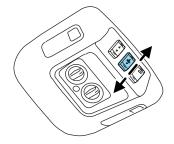
Press the  $\blacktriangle$  portion of the VENT control to open the power rear quarter windows.
