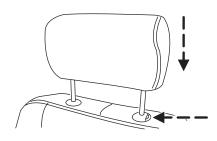
If the head restraint becomes detached, replace the notched bar into the bezel while holding the release button.
