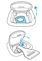
5. Clip the tether strap to the anchor as shown.
