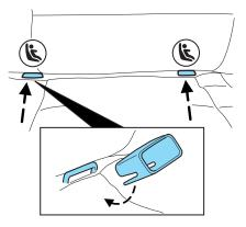
rigid attachments. The guides hold the seat trim away to expose the anchor and make it easier to attach some child seats.
