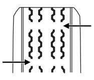
height as these "wear bars", the tire is worn out and must be replaced.
