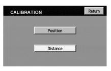
activate this function after every tire replacement. When the button is highlighted, calibration is in process and will turn off automatically when complete.
