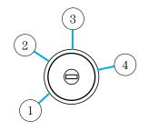
4. Within ten seconds of removing the previously programmed coded key, insert the other previously programmed coded key into the ignition.
