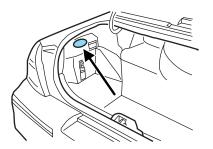
The fuel pump shut-off switch is located on a bracket inside of the luggage compartment.
