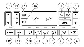
1. **A/C control:** Cools the vehicle and is used to reduce humidity in
