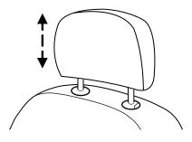
Push control to lower head restraint.
