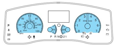
**Speedometer:** Indicates the current vehicle speed.
