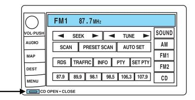
1. Press CD OPEN CLOSE at the bottom of the screen to load a CD. (The screen will open).
