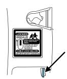
To open the luggage compartment door (lid) from within the luggage compartment, pull the illuminated "T" shaped handle and push up on the trunk lid. The handle is composed of a material that will glow for hours in darkness following brief exposure to ambient light.
