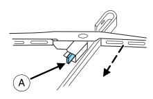
2. Attach the new blade to the arm loop and pull it into place until a click is heard.
