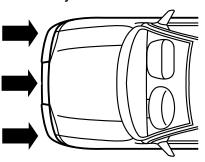
cause activation. Driver and passenger airbags are designed to inflate in frontal and near-frontal collisions, not rollover, side-impact, or rear-impacts unless the collision causes sufficient longitudinal deceleration.
