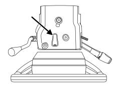
3. Remove the access plug using a flat head screwdriver, then push and hold the override button using a flat head screwdriver. Apply the brake pedal and shift the transmission into N (Neutral) while continuing to depress the override button.
