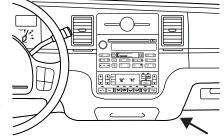
Do not hold the lighter in with your hand while it is heating, this will damage the lighter element and socket. The lighter will be released from its heating position when it is ready to be used.
