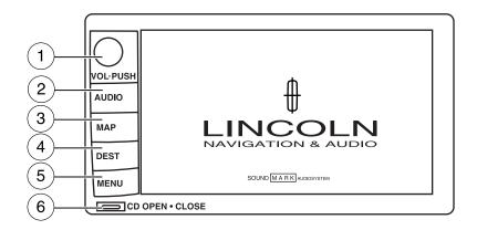
1. **VOL-PUSH**: Press to turn the system ON/OFF. Turn to adjust the audio volume level.
