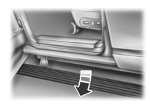
The running boards automatically move when the doors are opened to assist entering and exiting the vehicle.
