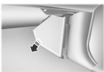
To remove the trim panel for access to the fuse box, pull the panel toward you and swing it out away from the side and remove it. To reinstall it, line up the tabs with the grooves on the panel, then push it shut.
