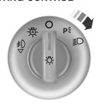
Rotate the control clockwise to the first position to turn on the parking lamps.
