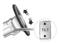
Use the control on the side of the steering column to tilt the position.
