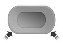
The control is located on the outboard side of the seat. Press the forward or rearward side of the control for more or less support.
