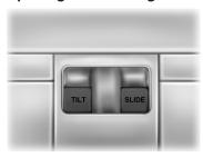
Press and release the **SLIDE** control to open the moonroof. The moonroof will stop short of the fully opened position.
