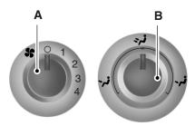
Your auxiliary climate controls are located on the rear of the center console and can be used when REAR has been pressed on the front climate control system. The temperature is set by the front controls. Use the rear control to adjust the fan speed or turn the auxiliary controls off (O).
