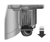
2. Unlock the locking clip on the connector (connector shown from below for clarity), then squeeze and pull the connector off of the air outlet tube.
