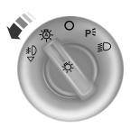
The autolamp system provides light sensitive automatic on/off control of the exterior lights normally controlled by the headlamp control.
