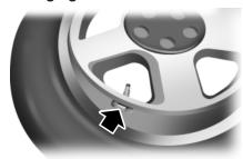
**Note:** Each road tire is equipped with a tire pressure sensor located inside the tire and wheel assembly cavity. The pressure sensor is attached to the valve stem. The pressure sensor is covered by the tire and is not visible unless the tire is removed. Care must be taken when changing the tire to avoid damaging the sensor.
