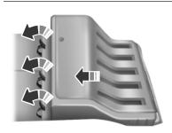
5. Release the three clamps that secure the cover to the air filter housing. Push the air filter cover toward the center of the vehicle and up slightly to release it.
