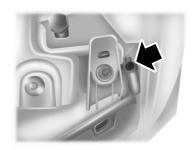
5. Locate the vertical adjuster on each headlamp, then use a Phillips #2 screwdriver to turn the adjuster either counterclockwise or clockwise in order to adjust the vertical aim of the headlamp. The upper edge of the light pattern should touch the horizontal reference line.
