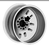
**Note:** Inspect the wheel pilot hole and mounting surface prior to installation. Remove any visible corrosion or loose particles.
