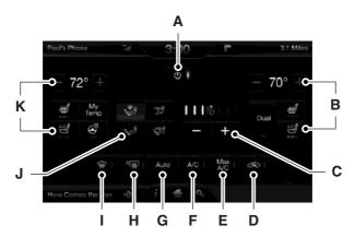
A. **Power:** Touch to switch the system off and on. Switching off the climate control system prevents outside air from entering the vehicle.
