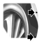
3. At the wheel well, remove the fasteners from the splash shield, then pull the splash shield back to gain access to the bulbs.
