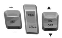
The cruise controls are located on the steering wheel.
