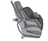
3. While holding the shoulder and lap belt portions together, route the tongue through the child seat according to the child seat manufacturer's instructions. Be sure the belt webbing is not twisted.
