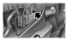
4. Locate the vertical adjuster on each headlamp. Using a Hex head driver, turn the adjuster either clockwise or counterclockwise in order to adjust the vertical aim of the headlamp.
