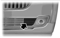
A message regarding a blocked sensor is displayed if the radar signals from the sensor have been obstructed. The sensor is located behind a fascia cover near the driver side of the lower grille. A vehicle ahead cannot be detected and the system will not function when the radar signals are obstructed. The following table lists possible causes and actions for this message being displayed.
