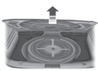
The system is located in the floor of the cargo area. Lift the release handle to open.
