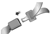
4. Insert the belt tongue into the proper buckle (the buckle closest to the direction the tongue is coming from) for that seating position until you hear a snap and feel the latch engage. Make sure the tongue is latched securely by pulling on it.
