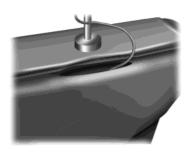
When in use, place the rear outboard safety belts in the comfort guides. These guides are attached to the head restraint and are stored in a pocket in the seat back.
