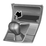
1. Using a screwdriver (or similar tool), carefully pry off and remove the Brake shift interlock access panel.
