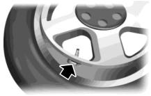
**Note:** Each road tire is equipped with a tire pressure sensor located inside the tire and wheel assembly cavity. The pressure sensor is attached to the valve stem. The pressure sensor is covered by the tire and is not visible unless the tire is removed. Take care when changing the tire to avoid damaging the sensor.
