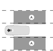
BLIS® aids the driver in detecting vehicles that may have entered the blind spot zone (A). The detection area is on both sides of the vehicle, extending rearward from the exterior mirrors to approximately 10 feet (3 meters) beyond the bumper. The system alerts you if certain vehicles enter the blind spot zone while driving.
