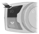
The fog lamps can be turned on when the lighting control is in the headlamps, parking lamps or autolamps positions and the high beams are not turned on.
