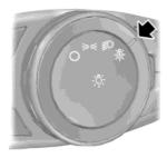
Note: If your vehicle is equipped with autolamps, it will have the windshield wiper activated headlamps. The windshield wiper activated headlamps turn on within 10 seconds when you switch the windshield wipers on and the lighting control switch is in the autolamps position. They will turn off approximately 60 seconds after you switch the windshield wipers off.
