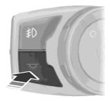
Use to manually turn the dome lamp on.
