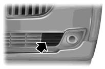
If a message regarding a blocked sensor appears in the information display, the radar signals from the sensor have been obstructed. The sensors are located behind a fascia cover near the driver side of the lower grille. When the sensors are obstructed, a vehicle ahead cannot be detected and the collision warning system does not function. The following table lists possible causes and
