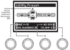
The **Signal Flow View** shows you all the amp and effects model "blocks" in your signal chain. From this view you can edit or move any component affecting your tone in the signal path. Use the **4 Way Nav Pad** to select an Amp, FX, or Looper block. At the bottom of the Signal Flow View screen, as well as in most other screens, you'll see up to four parameters that are accessed using the **Multi-Function Knobs** - these parameters are specific to the currently selected Block.
