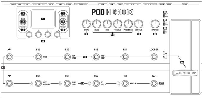
Display - The LCD is your window into the power of the POD HD500X.
