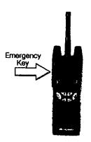
To make the call press and hold the key for more than 2 seconds. The behaviour of the unit after pressing the key depends on its personality programming.
